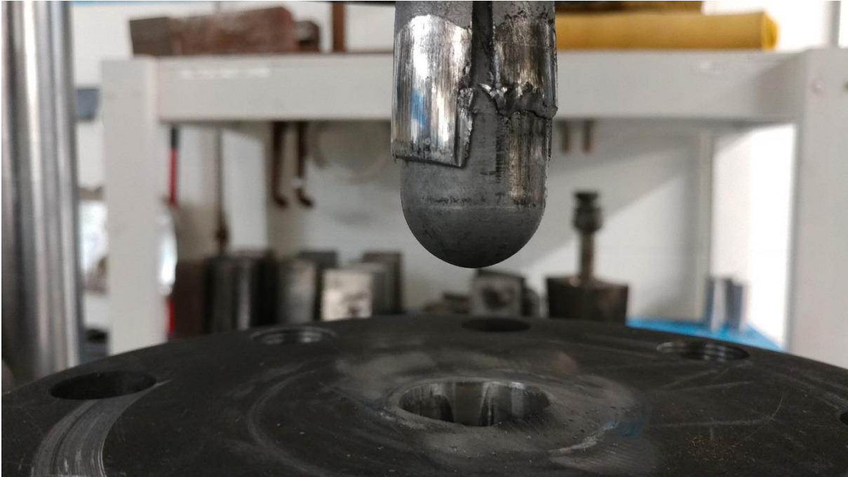
Figure 4: Tension Test 2 (180 ft lb installation) after testing
