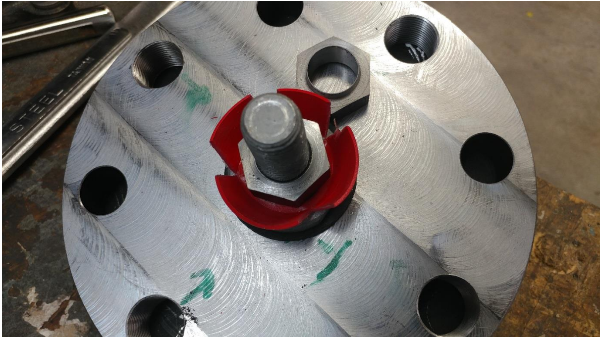
Figure 2: Tension Test Specimen after installation (nut shown sheared at 120 ft lbs)
