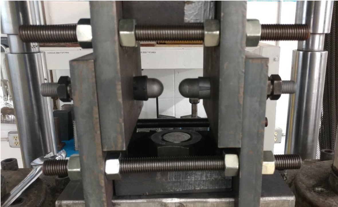
Figure 6: Shear Test Specimens installed before testing
