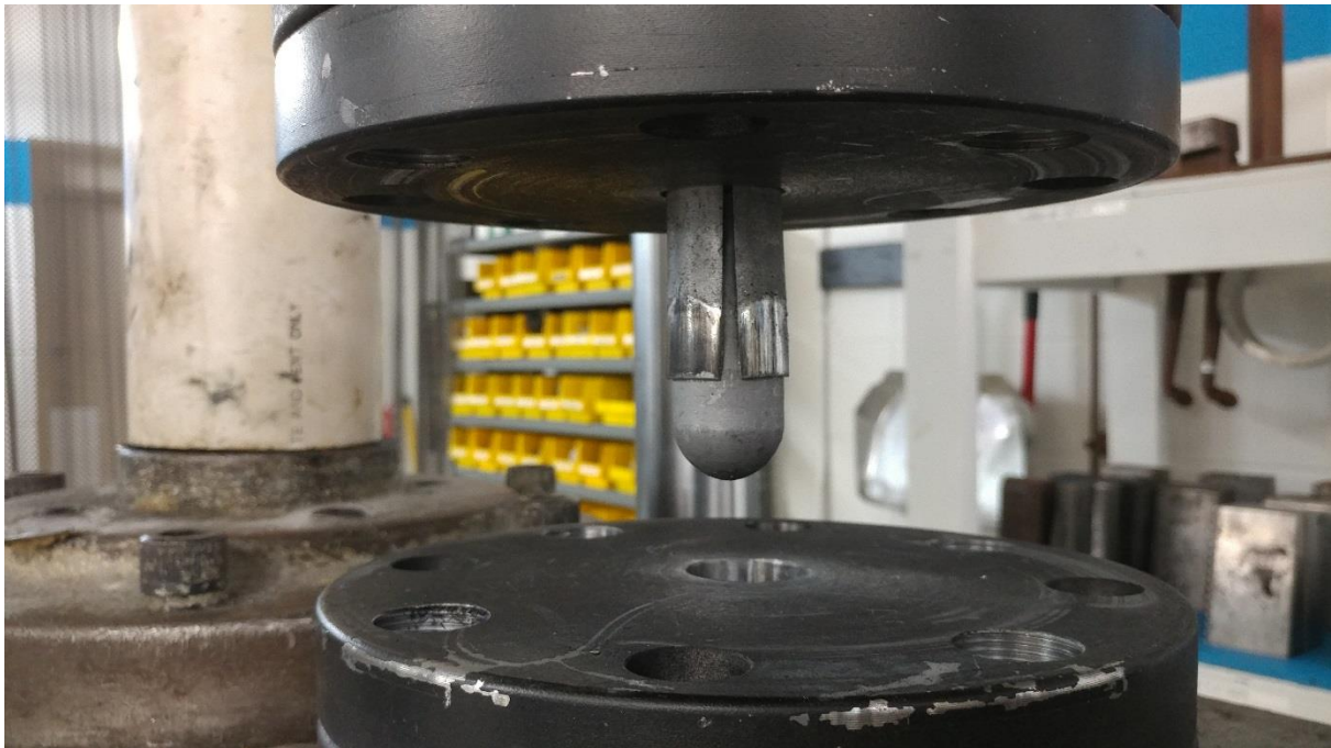
Figure 3: Tension Test 1 (120 ft lb installation) after testing
